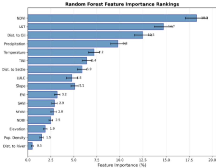
Fig. 3: Importance of features of the random forest model ranked in terms of mean decrease in Gini impurity.
